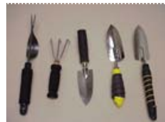
Figure No. 5: Tool handles with padding added to grip Source: University of Missouri
