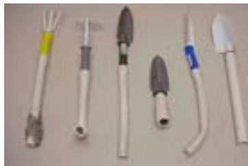
Figure No. 4: PVC added to tool handles Source: University of Missouri
