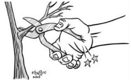
Poorly-designed tool: Handle presses into base of palm and requires user to open after each cut (no spring).
