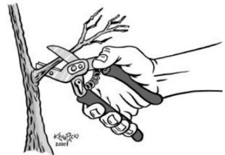
Well-designed tool: Handles are long. Spring return keeps tool open. Handles are covered with rubber or plastic grip.
